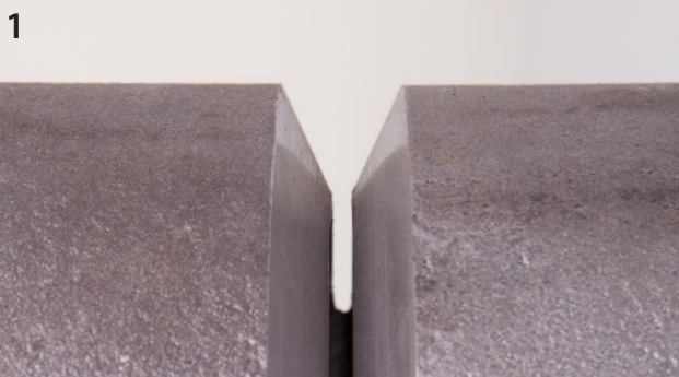
Weld preparation of root welds on pipes, 60° included angle with 3 mm air gap
