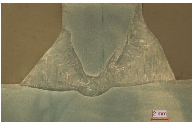
PB Full penetration, welded on both sides
