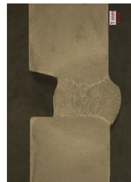
Material thickness 10 mm, one-sided bevel 15 degrees, air gap 4 mm
