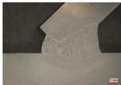
Web plate material thickness 10 mm, included angle 35°
