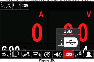
Press the Right Knob [36] to confirm the selection – the USB menu is shown on the display.
